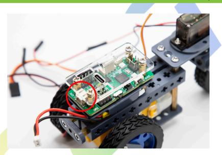
Ensure the battery pack wire and power port on the microcontroller are both facing the back of Motomo to allow for plug-in ease.
