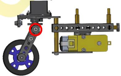
Ensure the headlight is facing forward. The front tire angle is adjustable at the indicated screw.
