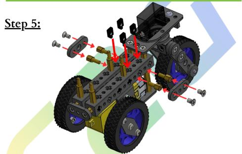
Place 4 black spacers into the top of the chassis blocks vertically, then insert 4 brass spacers tow on each side of the chassis, and secure the plastic footholds with two counter-sunk screws on each side all found in
